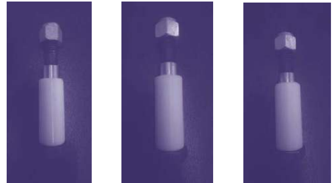
Fig. 15: Assembly of shackle pin and leaf spring plastic bush
