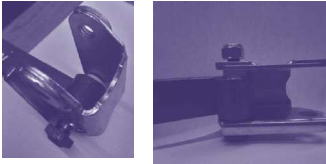
Fig. 14: Placement of bush in shackle as per its application
